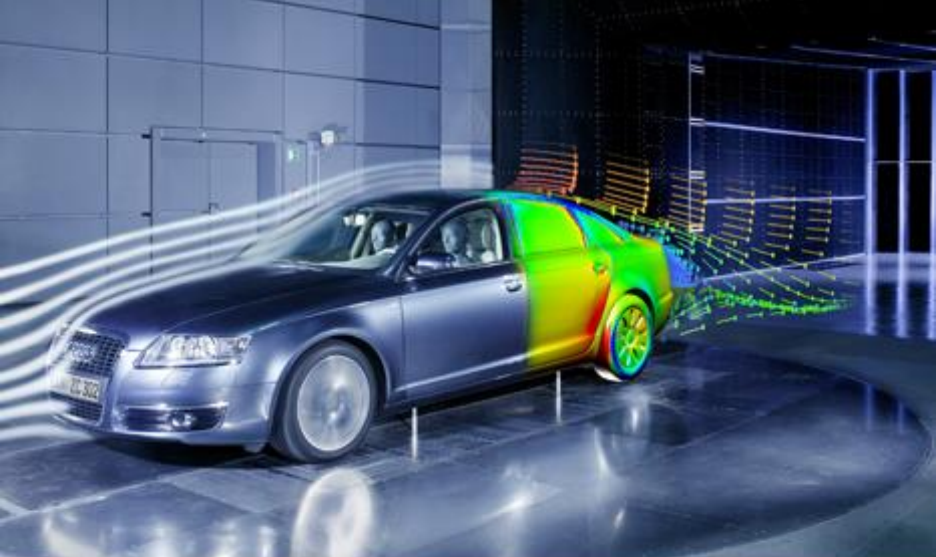
Wind tunnel smoke lines with CFD airflow superposed (credit AUDI Wind Tunnel Centre, 2013)
