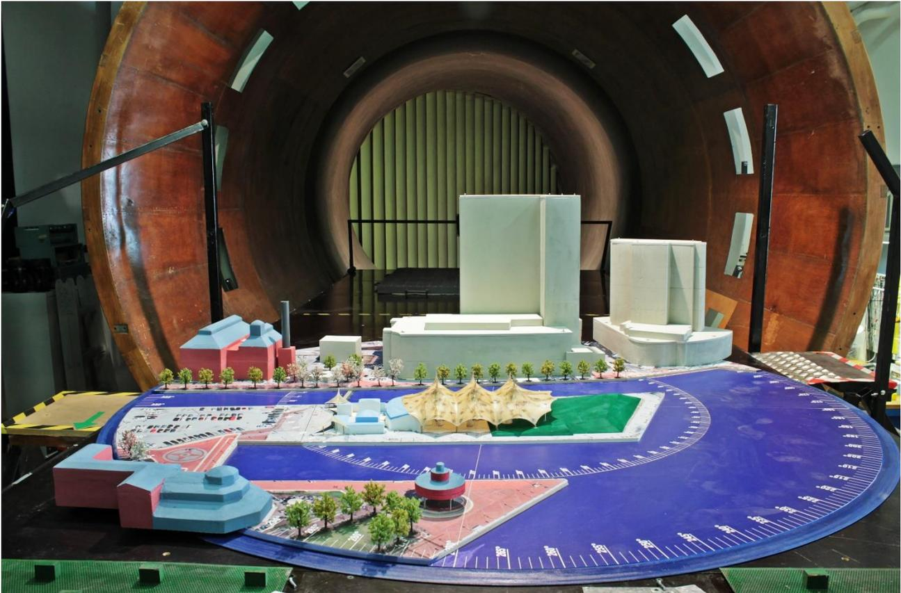
The wind tunnel model of a tensioned fabric structure and its surroundings (Baltimore, USA) in the existing wind tunnel of the Theodore von Kármán Wind Tunnel Laboratory of the Department of Fluid Mechanics at the Faculty of Mechanical Engineering of BME.
