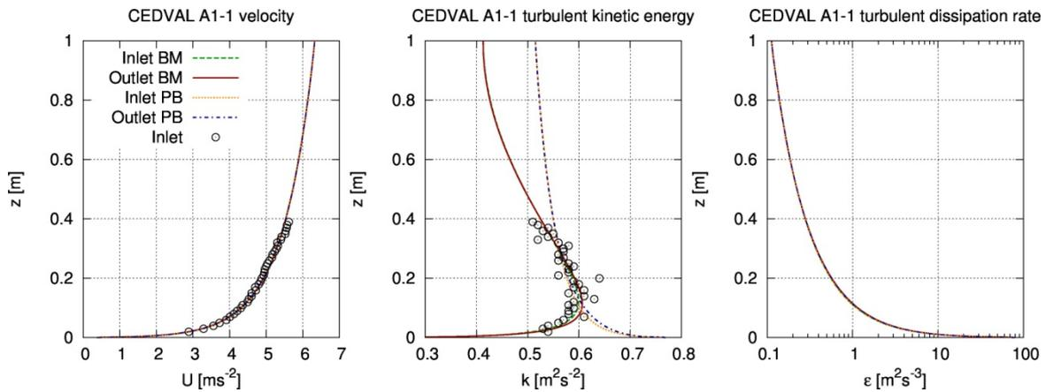
Figure 2: Inlet and outlet profiles against measurements for CEDVAL A1-1 case (PB. – Parente et al. 2011a, BM. – extended formulation).
