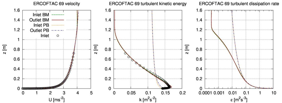
Figure 2: Inlet and outlet profiles against measurements for ERCOFTAC 69 case (PB. – Parente et al. 2011a, BM. – extended formulation).
