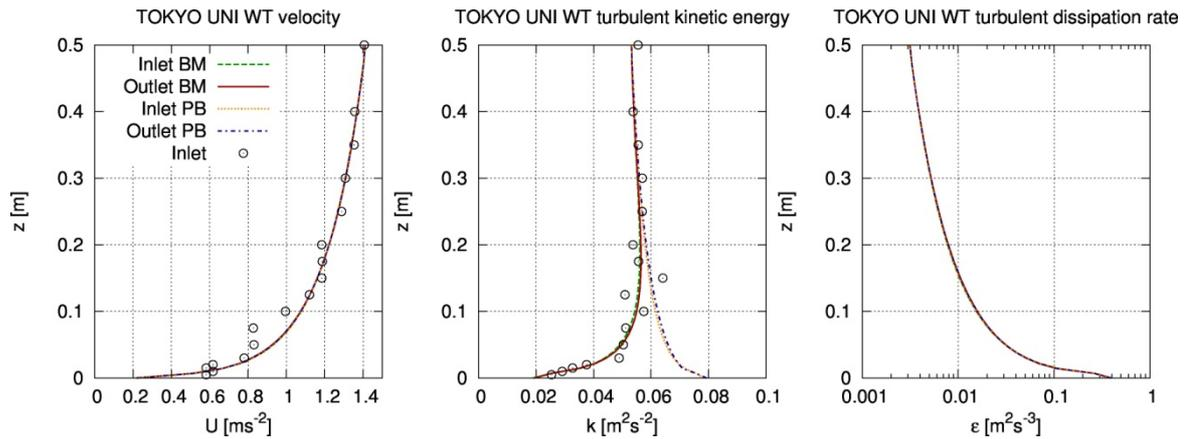
Figure 3: Inlet and outlet profiles against measurements for TOKYO UNI WT case (PB. – Parente et al. 2011a, BM. – extended formulation).
